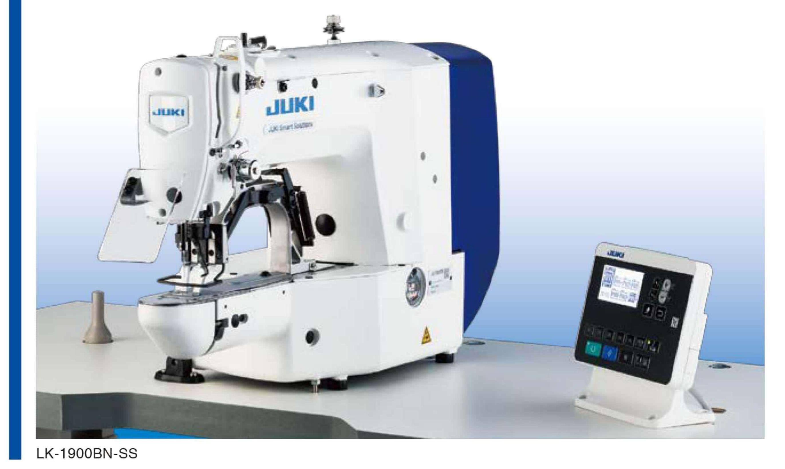
The machine achieves sewing speed of 3,200 sti/min The machine's threadtrimming etc. have been increased to significantly shorten total cycle time.
