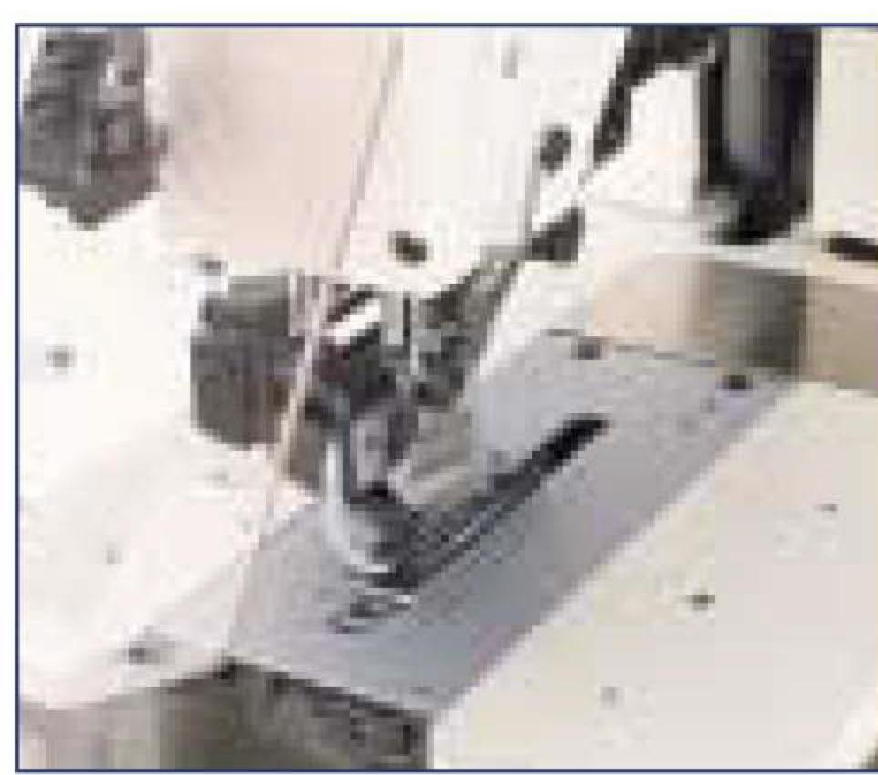
This needle entry point can visually checked. This permits easy positioning of buttonholes.
