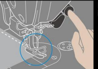
Easy reverse sewing operation with hand switch instead of reverse lever
